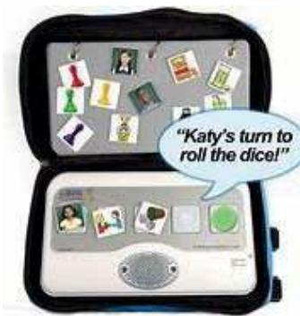
Proxtalker is the most advanced and adaptable recorded speech communication device available. It uses RFID (radio frequency identification) technology to enable independent verbal picture communication for non-verbal people of all ages. This technology allows you to simply place any photo, symbol, or object on a sound tag card and have a voice! To trigger voice output place your sound tag card on any one of the 5 buttons and push. Now silent picture users have easy access to voice output!
